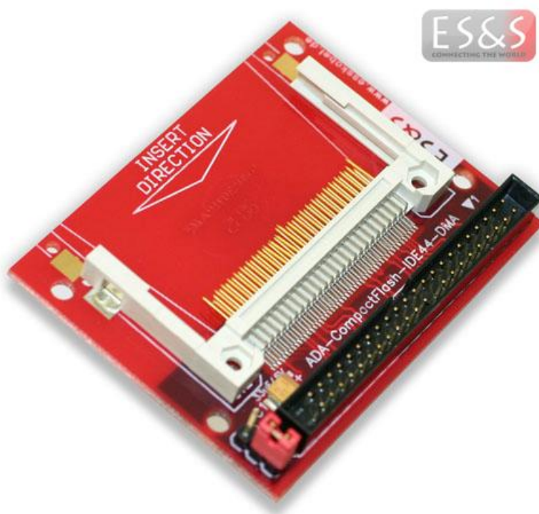
Compactflash to IDE44 adapter - short CF socket version
