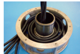
Small space wiring of twisting shaft
