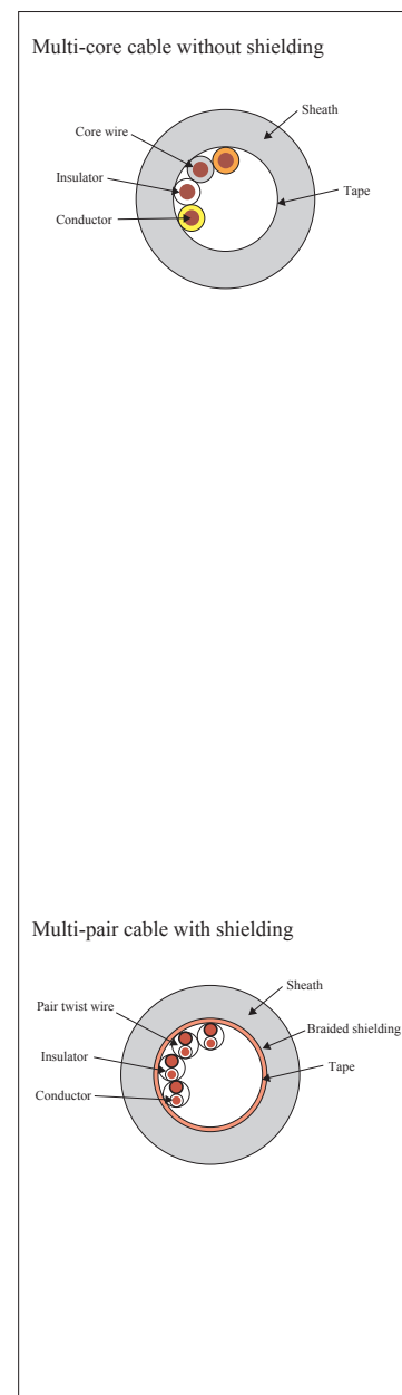
(Table 2) Configuration of multi-pair cable with shielding
