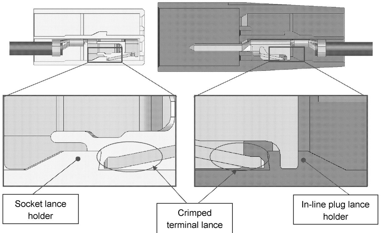
**\*Repair crimped terminals**
