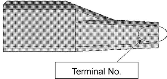
△ terminal numbers (Common to socket and in-line plug)
