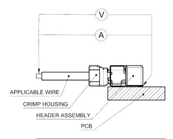
Contact Resistance:  $m\Omega = V/A$
