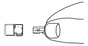
22. Please do not deliberately deform the movable portion (the lock area and lance of plug housing) and terminals. It would lead to product failure.
